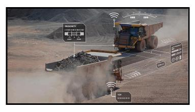
Another of their innovations is Collision Avoidance Systems (CAS)<sup>[35]</sup>. CAS comprises varying components that work together to remove the chance of human error, reducing injury and increasing profits. CAS is often used in transporting vehicles resources such as coal at mine sites. These components include live camera feeds, delineators (alongside roads site) and sensors with on
